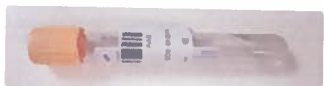
The 'I like it around the middle' specimen The bar code scanner on the analyser cannot read around bends. Would fail to be analysed. Builds delay.
