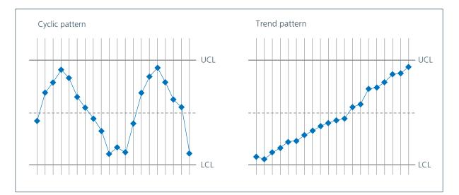
**Figure 5: Rule 4** – the number of points within the middle third of the region between the control limits differs markedly from two thirds of the total number of points:
